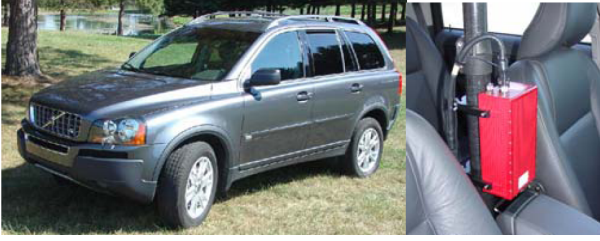
Fig. 6. The Volvo XC90 test vehicle with GPS system (Phanomchoeng et al. , 2011)
