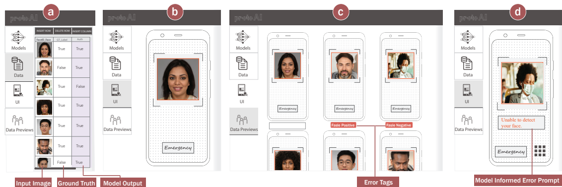
Fig. 1. Prototyping a Face-ID Phone Unlock user interface. The designer (a) provides a set of portrait photos and runs the Face-ID model, (b) prototypes the interface using a design-by-instance approach; (c) ProtoAI generates instances of the interface for all of the photos and flags false positives and false negatives. The designer (d) updates the design to include a numeric keypad and shows error message based on AI model output.
