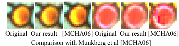
Figure 12: For an HDR image, aggressive tree compression in \log(\text{RGB}) space (at 1 bit/pixel), with remaining detail represented as a low-dynamic-range DXT1 image (4 bits/pixel). In comparison, Munkberg et al [MCHA06] report \text{rmse}=0.25 at 8 bits/pixel.
