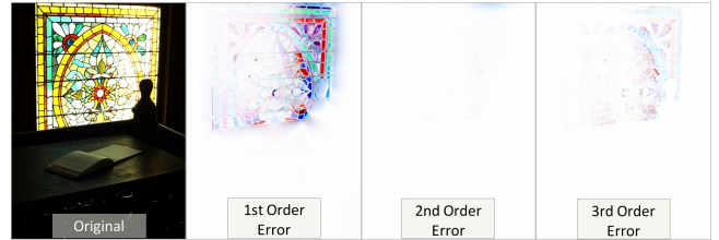
Figure 6: Visualization of the reconstruction errors for elements of order n=1,2,3 after a single V-cycle and k=2 Gauss-Seidel updates.
