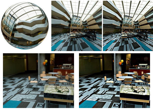
Fig. 12. Gradient-based sharpening on a gigapixel spherical panorama, computed in 136 seconds on a 4-node cluster.
