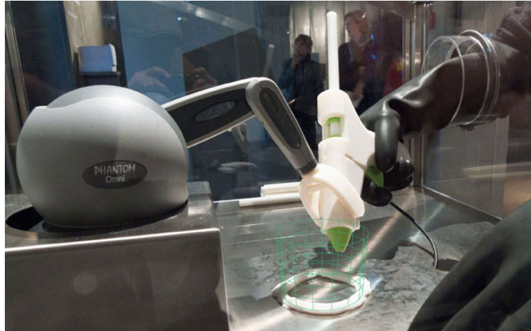
Figure 4.13: Continuous interactive fabrication by replicating an existing model: (a) Haptic Intelligentsia [Lee, 2011].
