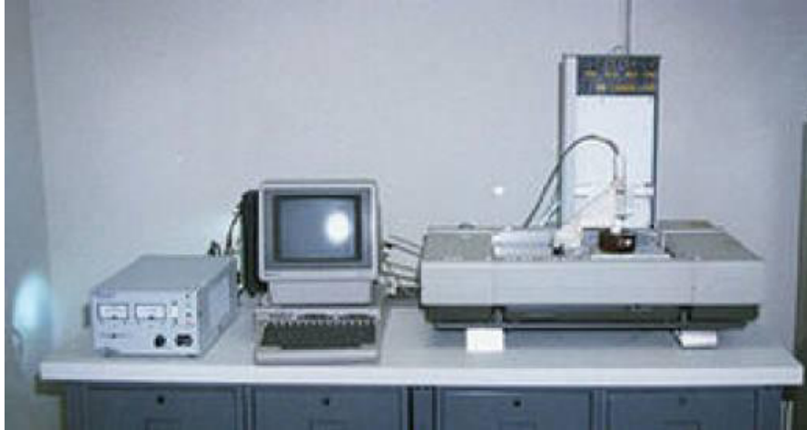
Figure 1.1: The first 3D printer: The SLA-1 from 3D Systems .
