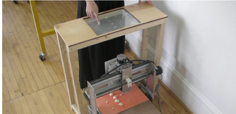
Figure 4.9: A touch on Shaper's [Willis et al., 2011] touchscreen causes the extruder to create a foam drop at the corresponding location.
