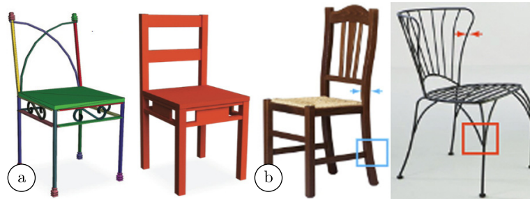
Figure 5.14: Mesh2Fab [Yang et al., 2015] preserves an object’s function by adapting the model geometry based on the available material.
