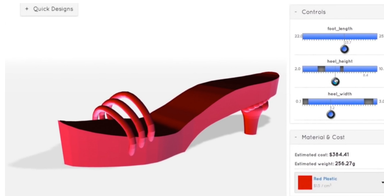
Figure 3.14: Parametrized Fab Forms [Shugrina et al., 2015] allow exploring only the physically valid options.
