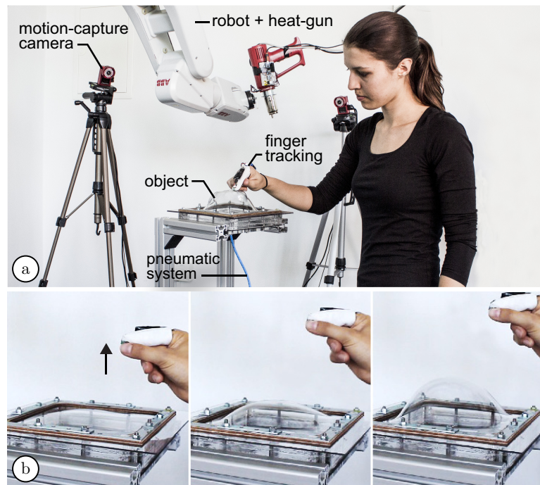
Figure 4.15: Continuous interactive fabrication: FormFab [Mueller et al., 2017] allows users to push and pull the material while receiving continuous feedback about the current state.
