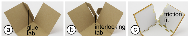
Figure 4: Traditional tabs (a) require gluing or (b) skillful insertion into the opposite tab. (c) Finger hinges, in contrast, stay put based on friction, eliminating the need for tabs.
