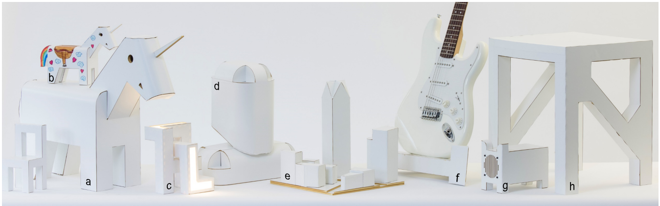
Figure 2: HingeCore objects created using HingeCoreMaker are not only fast to assemble, but also surprisingly sturdy. This allows building structural objects such as (a) toy horses, (f) guitar stands and (h) functional stools. HingeCore also offers a clean look, which allows creating (e) architecture models, as well as design objects, such as (c) lamps and (g) speakers. (b) The white exterior also invites coloring using art markers. The large unicorn and the stool were made from 10mm, all other models from 5mm foamcore.
