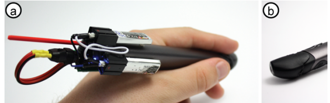
Figure 6: (a) Our second prototype was based on a hand-held extruder pen (3Doodler) retrofitted with a battery pack for mobile use. (b) We made an additional cap to allow users to put the device back into their pocket while still hot.
