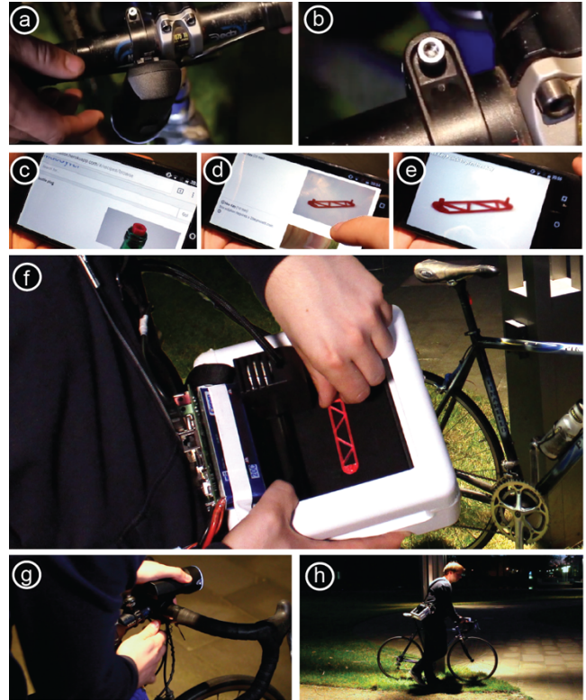
Figure 3: Walkthrough. (a,b) The user wants to go for a nightly bike ride. He finds that his bike lamp is sagging. Fixing it requires a hex key. (c,d,e) He opens our custom app to search for a solution. (f) He prints the solution on his portable 3D printer. (g,h) He fixes the lamp and rides off.
