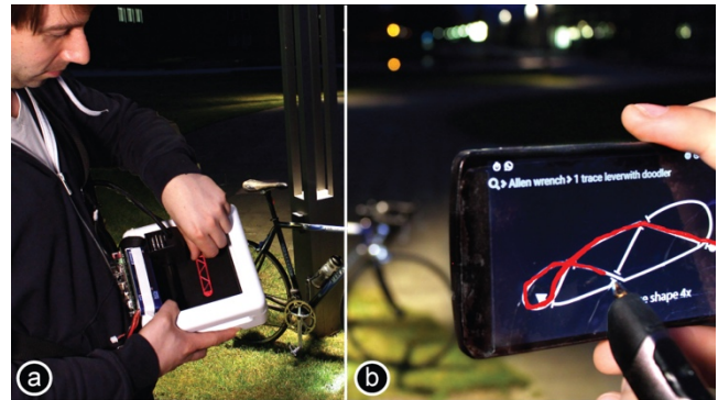
Figure 1: According to our survey, one use case of mobile fabrication is to fix things that break while on the go. This user, for example, fabricates a hex key to fix his broken bike light using either (a) a custom “mobile” 3D printer or (b) a “human-assisted” 3D printer based on an extruder pen. We drive both using a mobile phone running our custom app.
