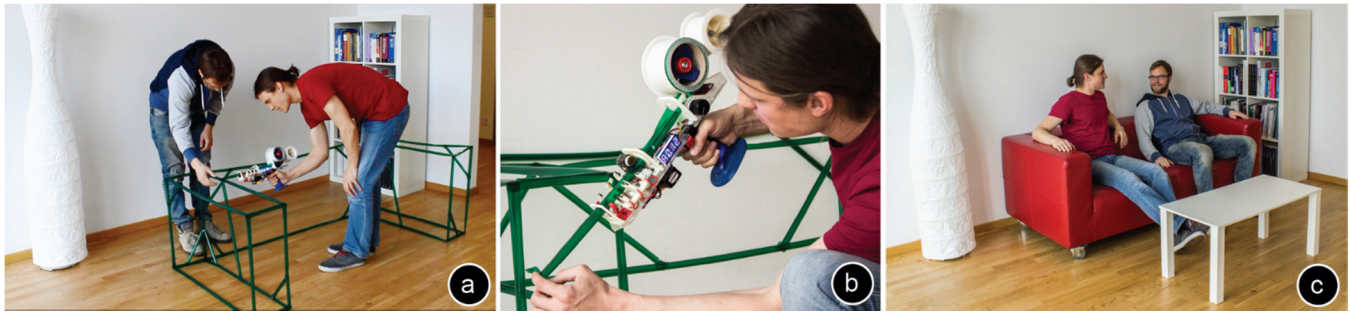
Figure 1: Protopiper is a hand-held physical sketching device. Unlike smaller devices that extrude plastic, protopiper creates tubes with connectors from adhesive tape. By allowing users to sketch and prototype room-sized objects at actual-scale, users can verify their designs during prototyping. For example, they can make sure that objects fit with the room or their bodies.
