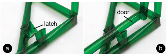
Figure 29: (a) Door latch in the shape of an “M”. The door’s weight allows it to latch into the “M”.
