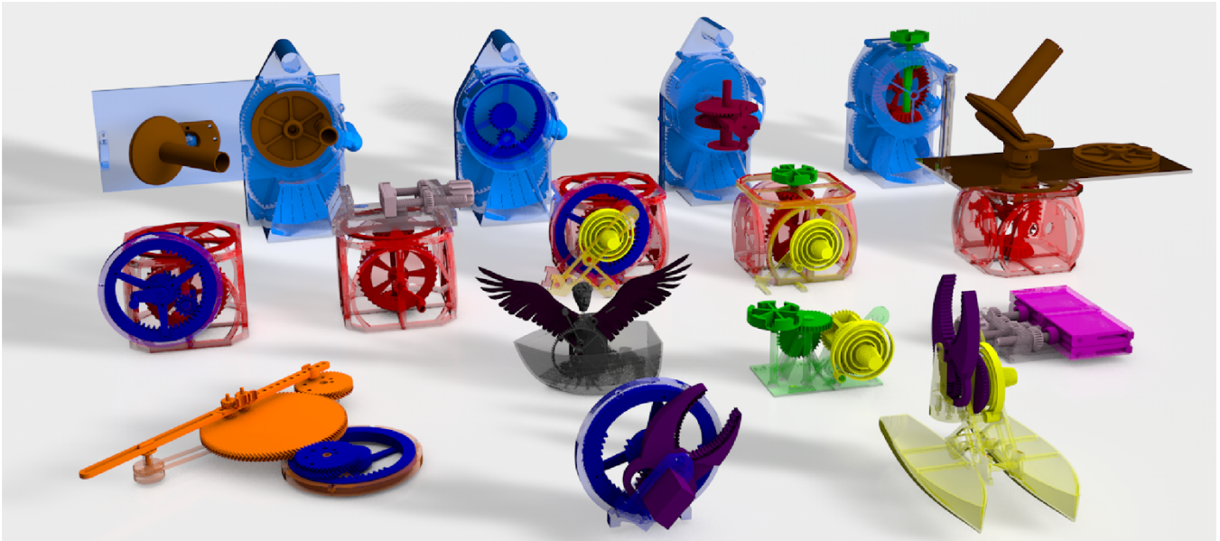
Figure 2: Some of the models we remixed using grafter , i.e., using mechanism-based remixing. Colors indicate the parent model from which the respective mechanism was taken. (a) All models in the top row are variations of the same actuation mechanism (a hand-cranked siren). (b) All models in the center row remix the same record player parent model, but replace different elements, i.e., actuation, transmission, or end effector. (c) Models in the front row sample a wider range of parent models.
