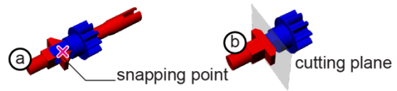
Figure 17: In order to merge the dragged mechanism into the target machine, grafter (a) overlaps the axles at the snapping point and (b) removes excess geometry.
