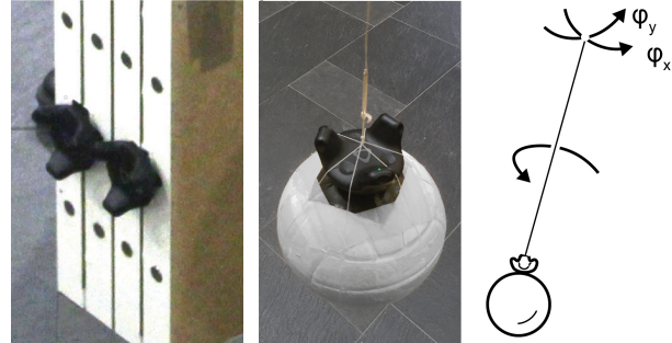
Figure 13: (a) Two Vive trackers allow the system to track the reconfigurable board in all its individual states. (b) The pendulum. (c) the state of the spherical pendulum is described by rotation angles on the pivot.
