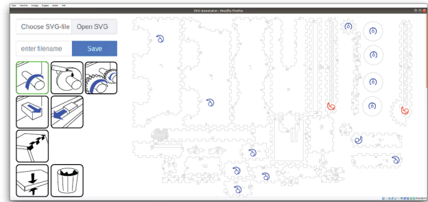
Figure 18: A model presented to the user (a firetruck). All outline geometry is greyed out to put the users’ emphasis on the mechanisms guessed by KerfCanceler.
