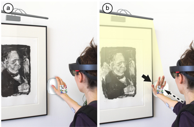
Figure 5: Turning on the virtual lamp. Here our EMS system renders the forces of the button’s mechanism.
