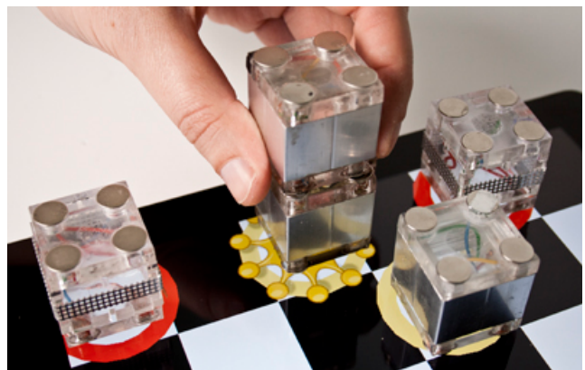
Figure 1: Enabling a game of tangible checkers, the capacitive touchscreen distinguishes a stack of two CapStones from the single CapStones surrounding it.
