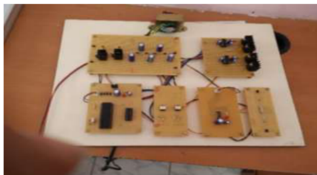
Figure 20 High Voltage DC-DC Converter
