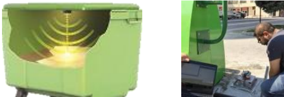
Figure 1. The placement of integrated sensor box inside the garbage containers.
