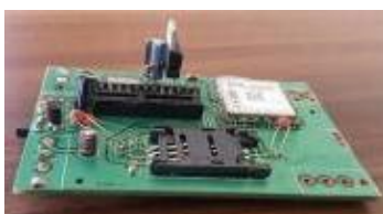
Figure 3. The integrated sensors box of micro controller and IoT cellular module.
