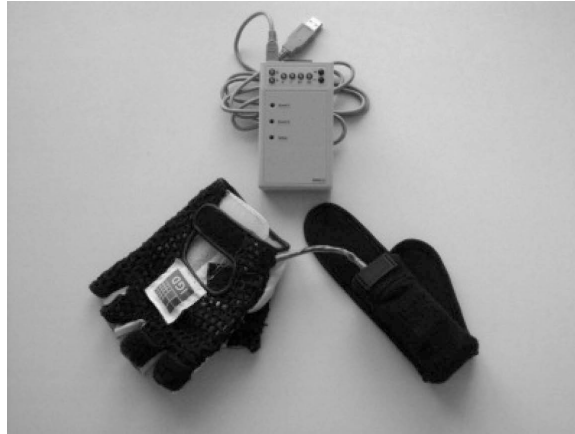
Fig. 16.3 In EREC-II, the sensing circuitry is accommodated by a wrist pocket, making the glove lighter and more airy. It also allows for more flexible system arrangements.
