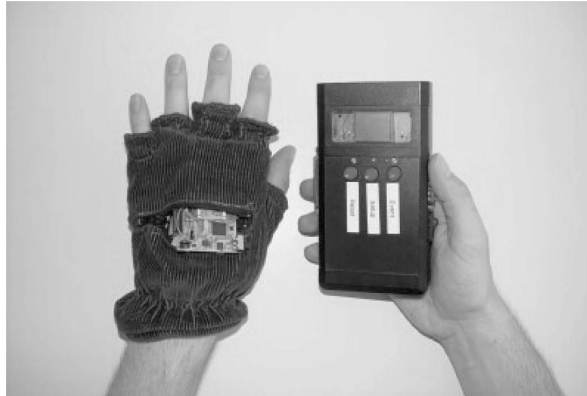
Fig. 16.2 The first prototype EREC-I consists of a glove hosting the sensor elements and the processing electronics, and the base unit with display, memory card, and serial port.
