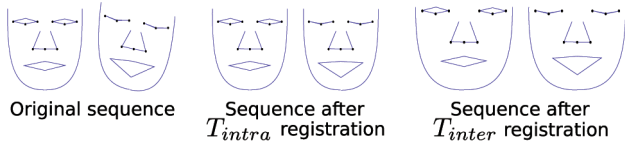
Fig. 3. An illustration of the rigid registration process. Also shown are the 10 facial feature points used for registration.
