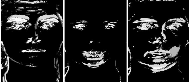
Figure 1. Motion History Images (MHIs) of activated Action Units AU1+AU2 (left), AU16 (mid) and AU36L (right)
