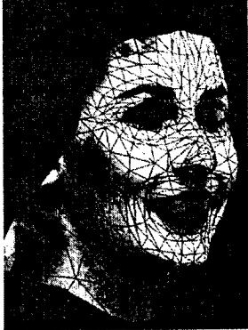
Figure 2.4: 3D mesh with texture mapped triangles proposed by Terzopoulos and Waters (1993)
