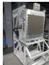
2010 5.8GHz, Total Power >1.9kW 256 array module HPA PAE >70% (GaN) thickness <30cm in Kyoto Univ.
