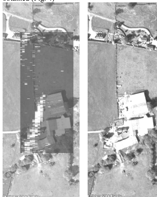
Figure 4: BSAR image of a building with Galileo as the transmitter and a moving ground vehicle as the receiver superimposed on a satellite optical photograph (a), optical photograph (b).
