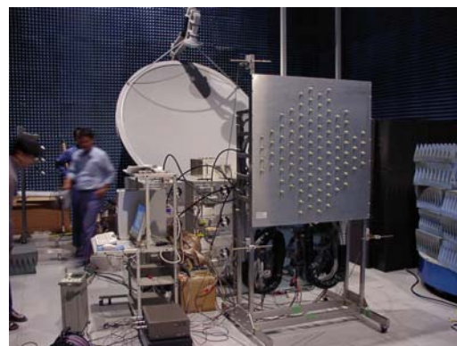
Figure 7 Magnetron Phased Array with Phase Controlled Magnetron through 1-bit sub-phase shifters after 8-way power dividers
