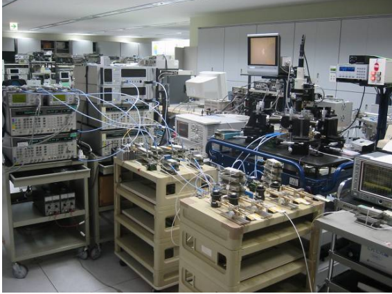
Figure 4: Experimental configuration for IMD measurement.
