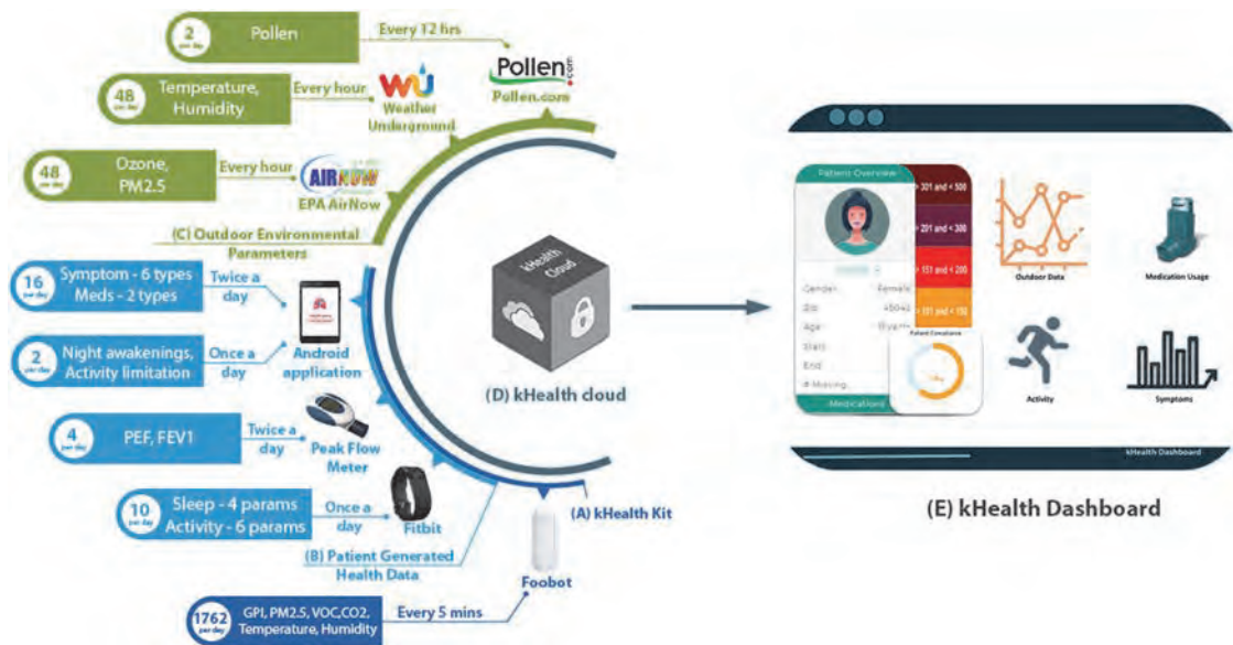
Figure 2. The kHealth framework with kHealth-Asthma kit, kHealth cloud (D), and kHealth Dashboard (E), showing the frequency of data collection, the number of parameters collected, and the total number of data points collected per day per patient (shown in dark blue). The kHealth kit components that are given to patients which collect PGHD are shown in light blue and the outdoor environmental parameters with their sources are shown in green. All data are anonymized and associated with respective randomly assigned patient IDs.
