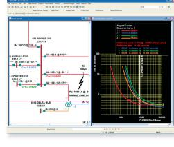
TCC display makes it easy to see how coordination time intervals change when you move the fault around.
