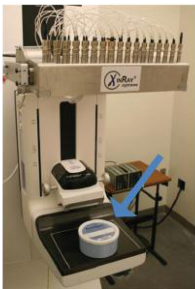
FIGURE 18. CNT based breast tomosynthesis system (reproduced with permission from [62]).
