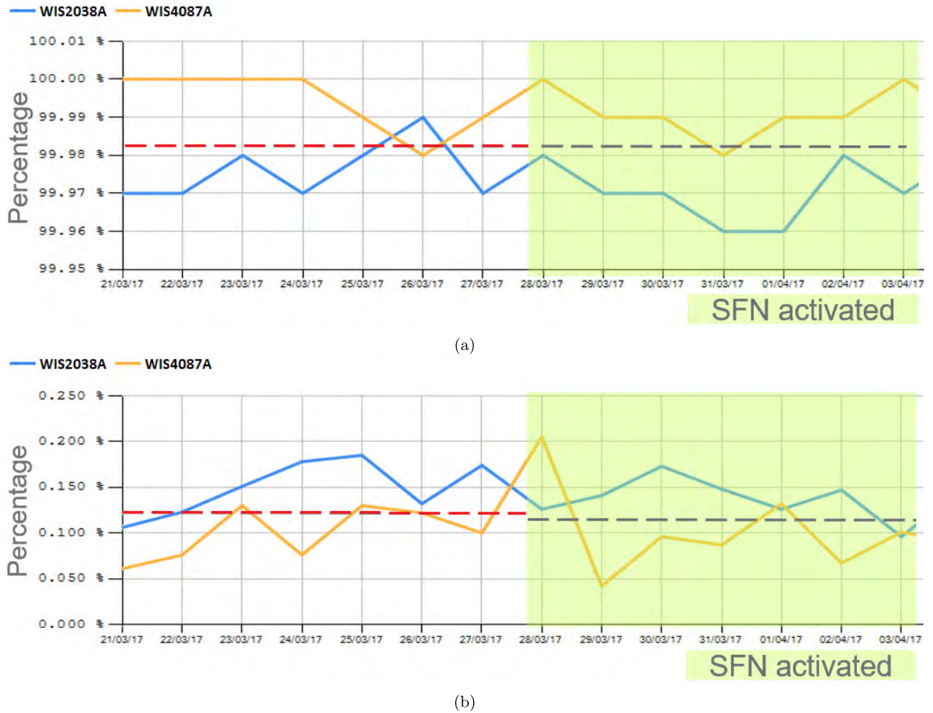
FIGURE 15. Single frequency network (a) RRC setup success rate (%). (b) Service drop rate (%).
