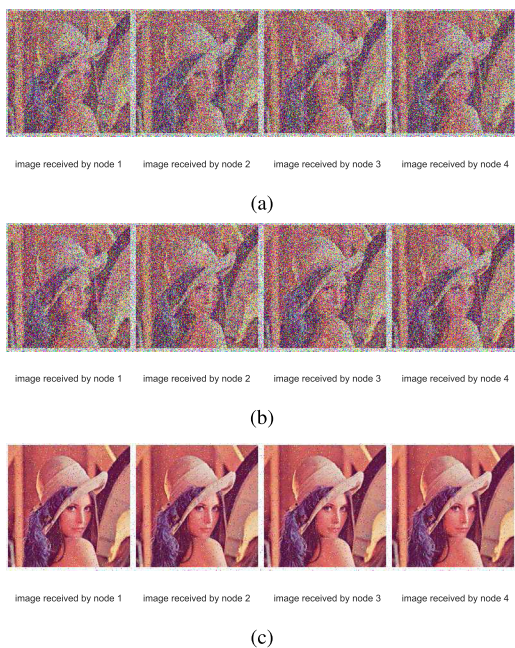
FIGURE 8. Anti-jamming effect of the ACA model with four nodes by loading three allocation methods. The jamming power is 2w , the system total power is 1w , and the number of subcarriers is 64. (a) Images received by 4 different nodes using random allocation method through OFDM system based on ACA model. The same image is sent by nodes at the transmitting end. (b) Images received by 4 different nodes using fixed allocation method through OFDM system based on ACA model. The same image is sent by nodes at the transmitting end. (c) Images received by 4 different nodes using JSER algorithm through OFDM system based on ACA model. The same image is sent by nodes at the transmitting end.
