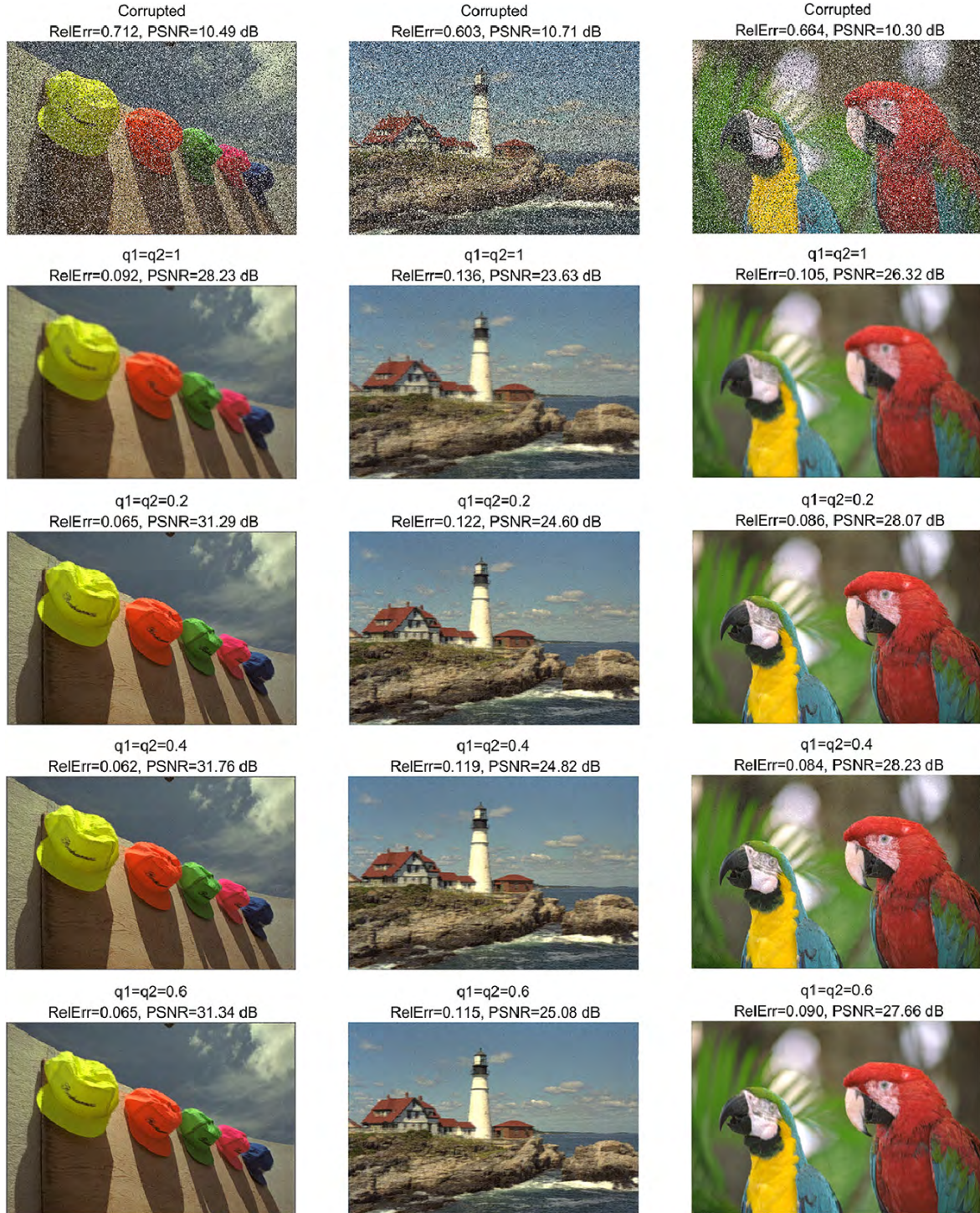
FIGURE 4. Recovery performance of the proposed algorithms on three 600 × 400 color images corrupted by salt-and-pepper noise.
