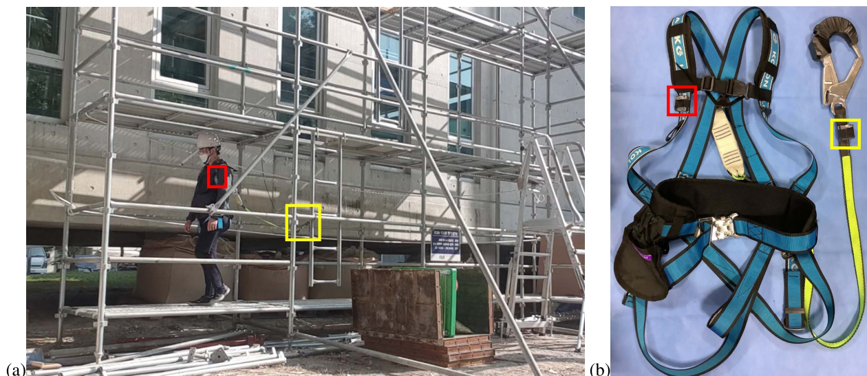
FIGURE 3. (a) Data acquisition in the construction site testbed. (b) One mobile device (Red box) is attached to the the chest strap of the safety harness and the other (Yellow box) is attached to the neck of the safety hook.
