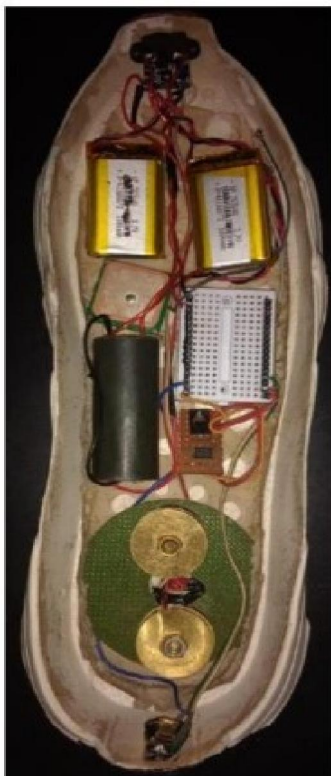
Fig.7: Shoe (Node MCU, Shockwave Generator, Buzzer, Battery).
