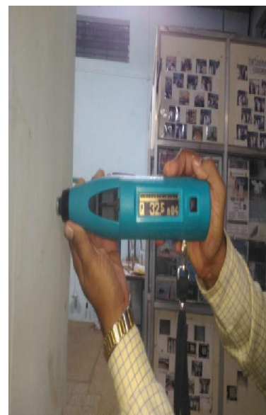
Fig. 4.2 : (c) Rebound Hammer test on Column and Beam
