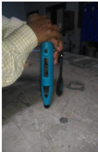
Fig. 4.2 : (b) Rebound Hammer test on slab
