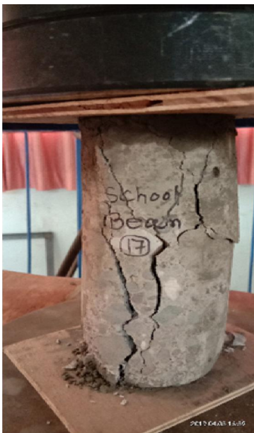
Fig. 4.2 : (a) Concrete Core Testing
