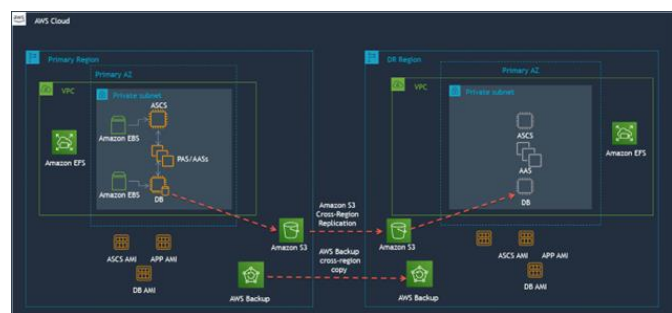
Figure 3 Passive Disaster Recovery for SAP applications using AWS Backup and AWS Backup Agent (AWS, 2021)
