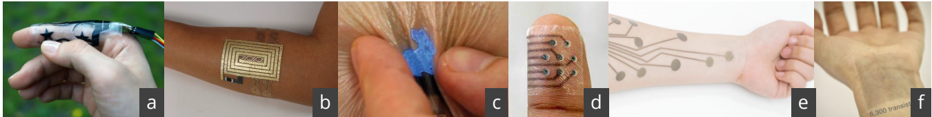
Figure 1: Examples of Epidermal Computing Devices for a) eyes-free touch input [230], b) wireless communication through aesthetic on-skin tattoos [97], c) displaying notifications through ultr-thin displays [232], d) feel-through haptics [234], e) sensing physiological signals [155] and f) skin stretchable large scale transistor array for on-skin computing [225]
