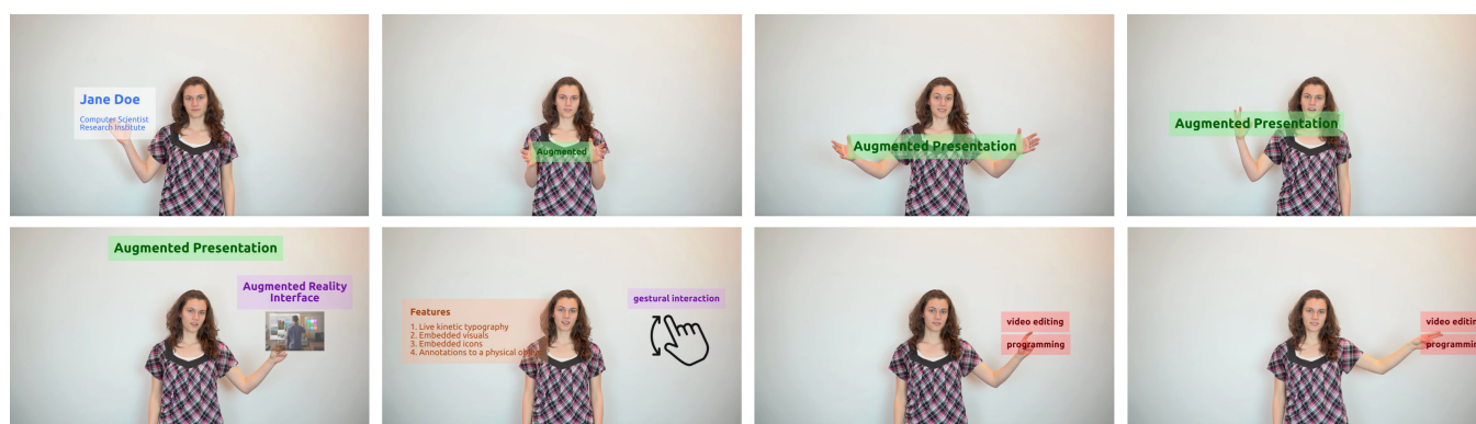
Figure 1: RealityTalk augments live video presentations with speech-driven interactions, where the live speech and supporting modalities (such as gestures) drive the triggering and manipulation of textual and graphical elements on the screen.
