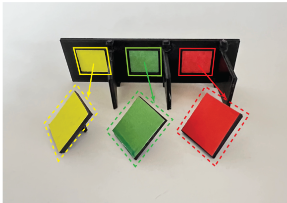
Figure 11: Selectively magnetic lock-and-key systems. Colored locks (solid lines) mate with keys of the associated color (dashed line), but not others.
