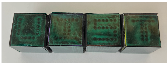
Figure 12: Selectively attractive faces between the cubes guide users into the correct assembly. The letters are plotted onto the top surface of the cubes and made visible with magnetic viewing film.
