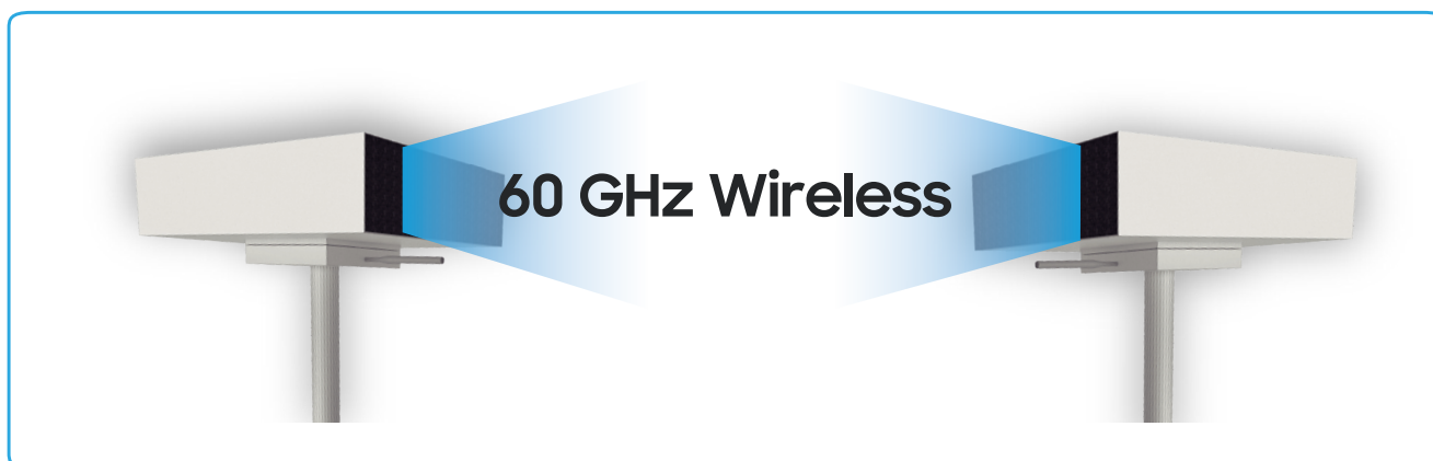
Figure A. mmWave Wireless Backhaul Concept
