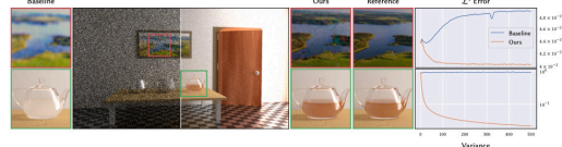
Fig. 1. We improve physics-based differentiable rendering by introducing a recursive control variate into the optimization loop. Left: A baseline method [Vicini et al. 2023] repeatedly renders noisy images to compute gradients. The noise leads to poor convergence. Right: applied on top of the baseline, our recursive control variate reduces the noise using information from similar renderings in prior optimization steps. This leads to a reconstruction that is much closer to the reference image. The plots show the evolution of the loss function and rendering variance as the optimization progresses.
