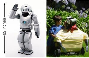
Left: QRIO, a prototype humanoid developed by Sony. Right: RUBI, a prototype humanoid developed at our laboratory.
