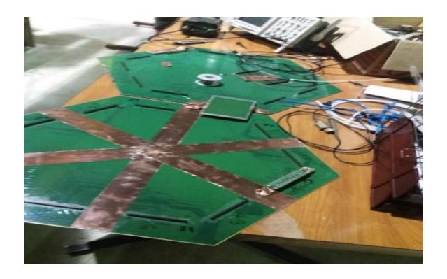
No signal loss was observed by injecting a signal on the furthest end of the first PCB and detecting it on the opposite side of the second one.
