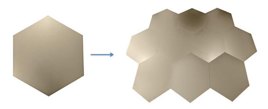
Large detection area can be instrumented by assembling easily many PCB.
