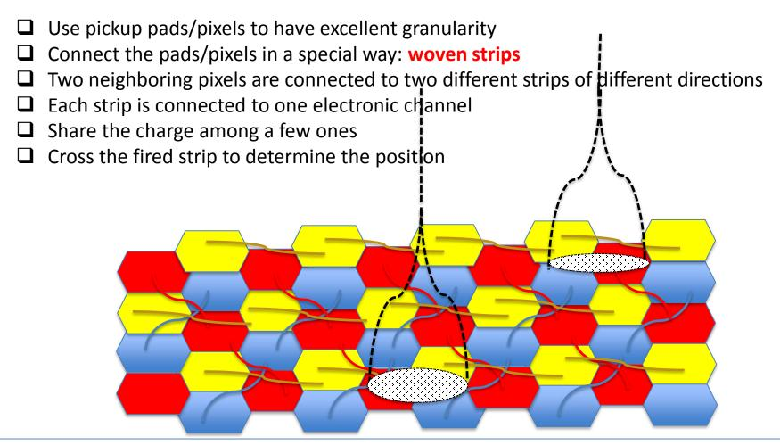
NXN  $\rightarrow$  3N : Reduction of electronic channels, power consumption and occupancy
