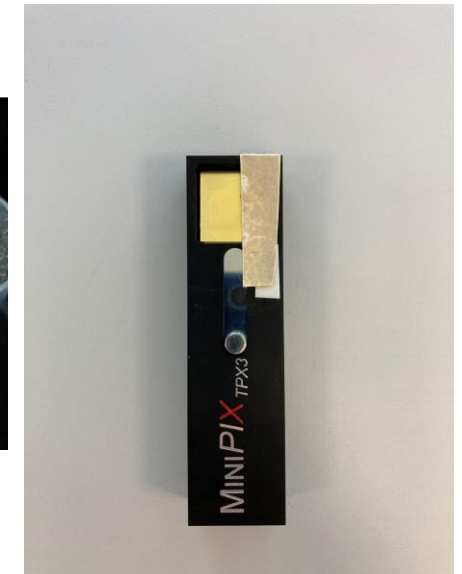
MiniPIX Timepix3 hybrid pixel detector with 4H-SiC sensor and sulfur layer applied
