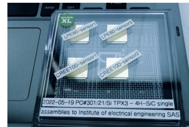
Prepared pixelated structure on 4H-SiC epitaxial layer.
