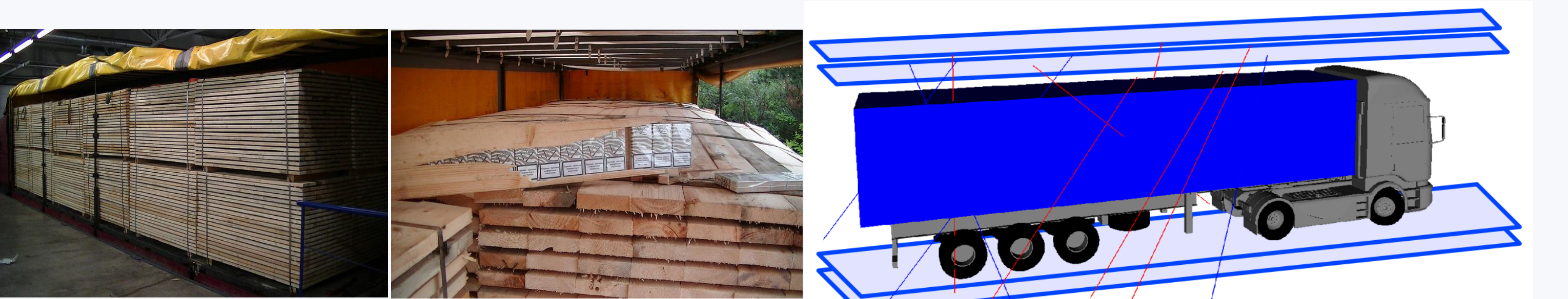
Fig. 11 Real cigarette smuggling to replace part of wooden boards. Fig. 12 Geant4 model of semi-trailer loaded with wooden boards.
