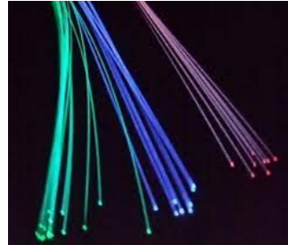
Plastic scintillator fiber (d = 1 mm)
