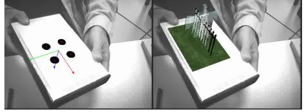
Fig. 4. Pose estimation using planar version of POSIT [93] followed by a non-linear estimation process [78] to improve the registration.
