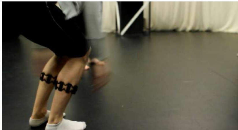
Figure 5.16. A participant interacting with the Still, moving installation. The Myo devices are capturing muscular activity and motion to generate the sound environment
