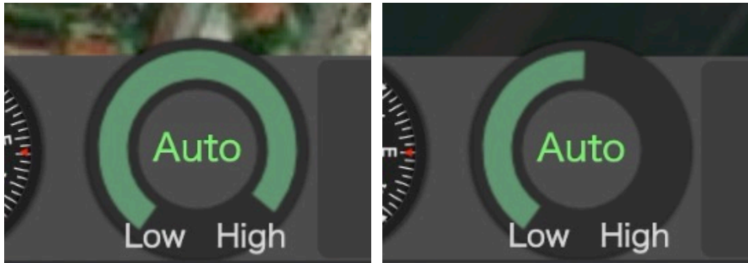
Figure 4.4: Reliability Indicator at the bottom left area of the screen. Showing a higher reliability (left) and a deteriorated reliability (right).
