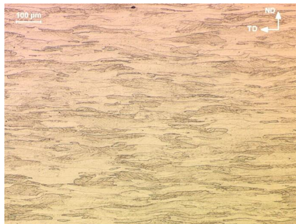
Fig. 8.3: Optical microscope observation of cold worked molybdenum.
