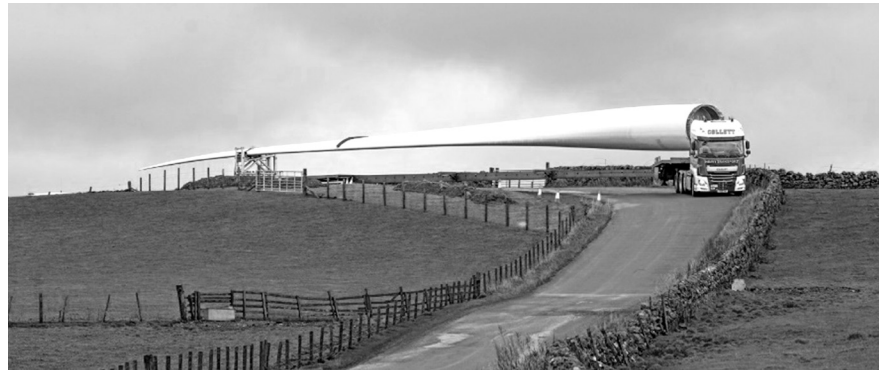
Fig. 1. UK's Largest Onshore Turbine Blades, transport to Muirhall Wind Farm, South Lanarkshire (Wikimedia Commons, 2019).
