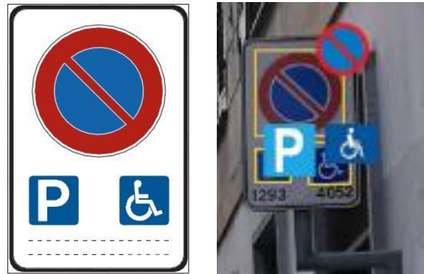
Figure 11. A standard traffic sign identifying a parking lot reserved to a disabled person (left) and how it is recognised by Mapillary algorithm (right)
