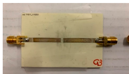
Figure 1. Prototype of the microstrip line with gap without film deposition.
