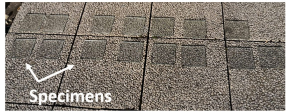
Fig. 4 Set of 15 coated glass specimens exposed to atmospheric agents
